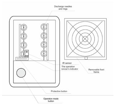
Bipolar air ionizer "Yantar 5A" is a desktop device. The most of front and rear panels are occupied by concentric grills. The air is sucked through the rear panel by the fan, and is blown away through the front panel.
