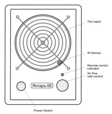
The frame and the grill on the front panel are detachable to allow easy dusting of needles and cleaning scurf. It's recommended to clean the needles in 2 steps.
