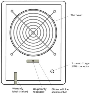
On the rear side, there is a control, which make it possible to set the required unipolarity factor. Adjustments to unipolarity factor cannot be made without the air ion counter, which gauges both polarities simultaneously.
