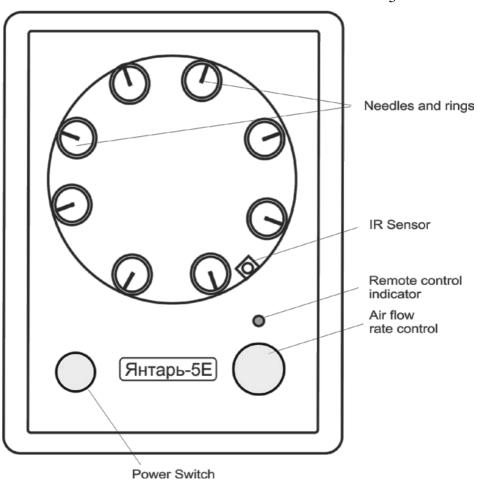
The operating voltage at needles can reach 4000 volts, so ensure the ionizer is switched off from the power mains before detaching the frame.
